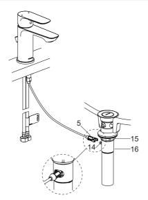
Install the cable end(5) into the magnetic snap(14), ensure the buckle is locked.
